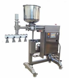
The electronic-volumetric depositor (DVE) has a pumping system with a syringe. The device is activated by a brushless motor and it's
